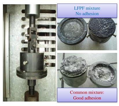
The device evaluating the adhesion property between ice and asphalt mixture
