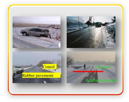
The de-icing ratio is up to 62%. The friction coefficient increased by 84%. The driving safety was improved.
